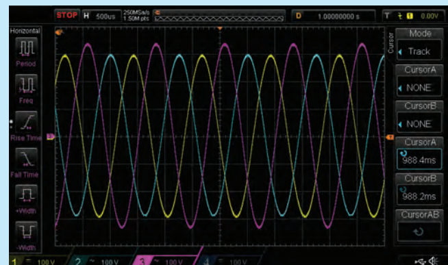
Three Phase Unbalance Voltage Test Captured
