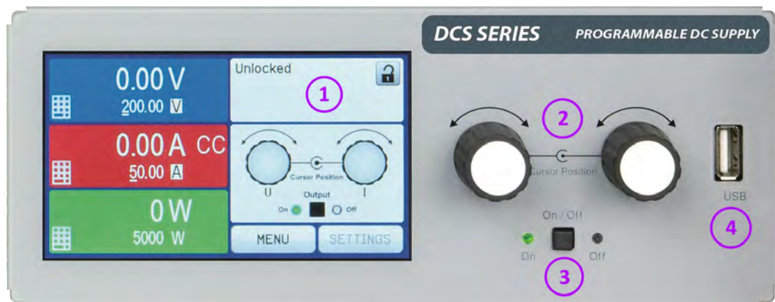
Figure 6-1: DCS Series Front Panel View
