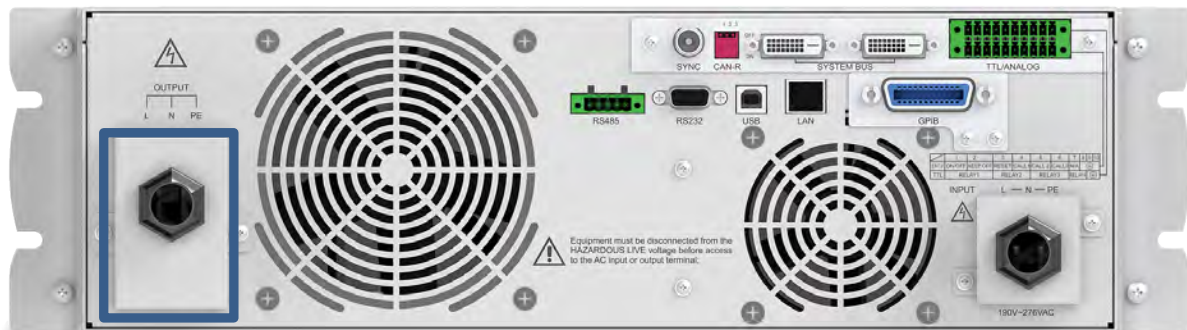
Figure 5-5: Output Terminal Locations - 3U Models
