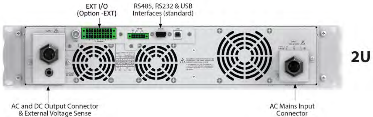
Figure 5-8: Rear Panel Callouts – 2U Models
